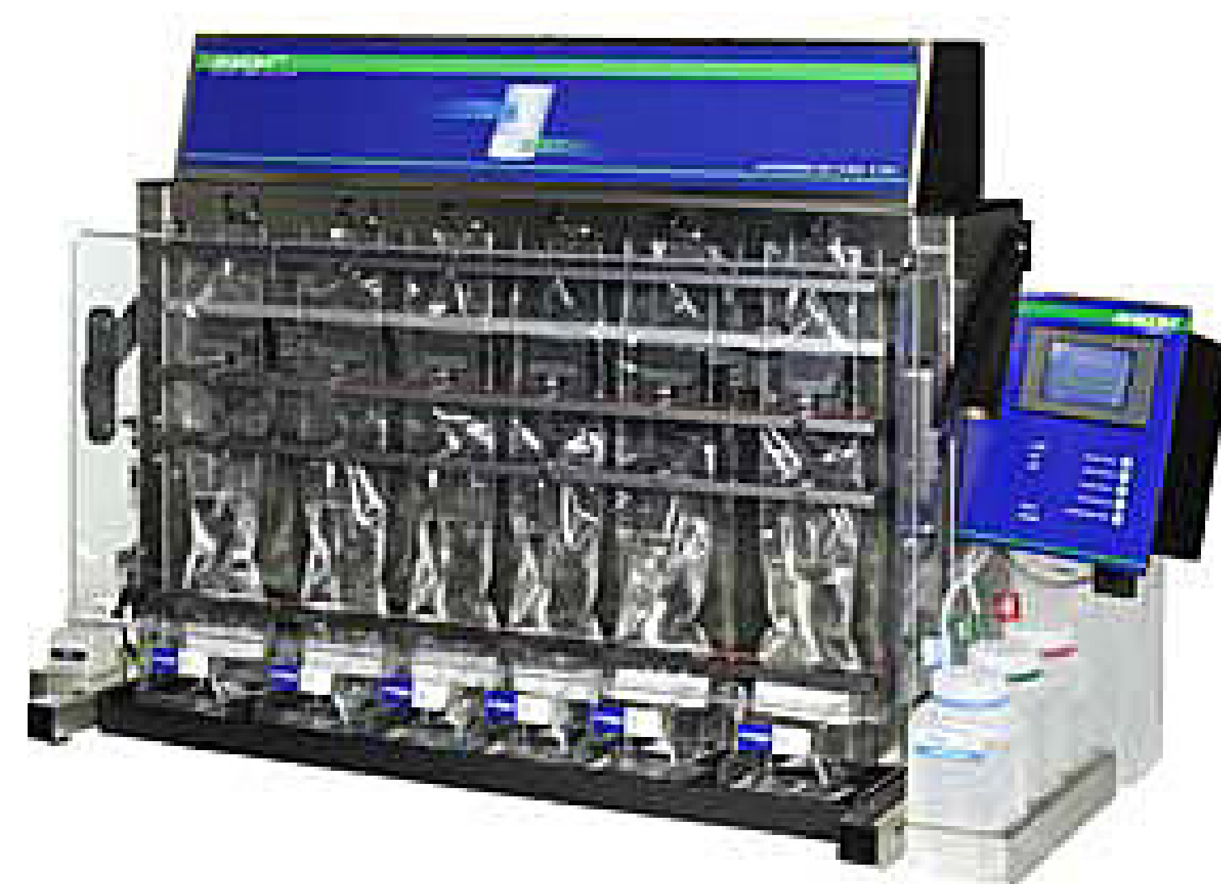
Figure 1. Dietary Fiber Instrument, Ankom™ Dietary Fiber Analyzer
